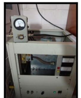
POWER AMPLIFIER USING EIMAC 8877
